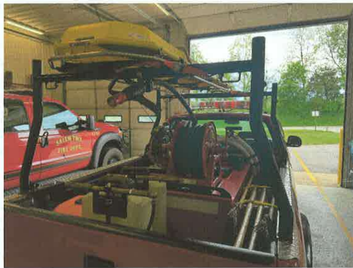
New Skid Unit- Pump/tank in 1731 with a ladder rack to carry the Stokes Basket.
